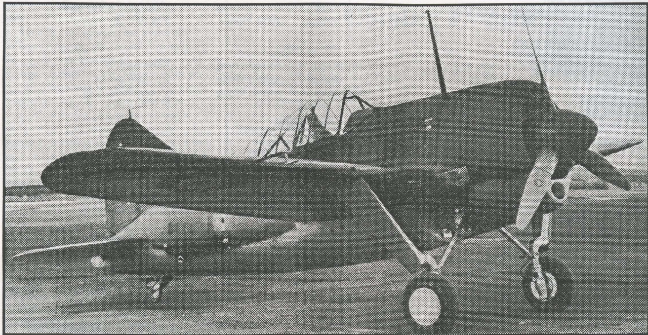
The Belgian Model 339B featured a pointed tailcone which lengthened the Buffalo's fuselage slightly. The carrier style tail wheel and cuffed Curtiss Electric propeller of the F2A-2 have been retained, but the pitot tube has been replaced by an 'L' shaped pitot tube.
